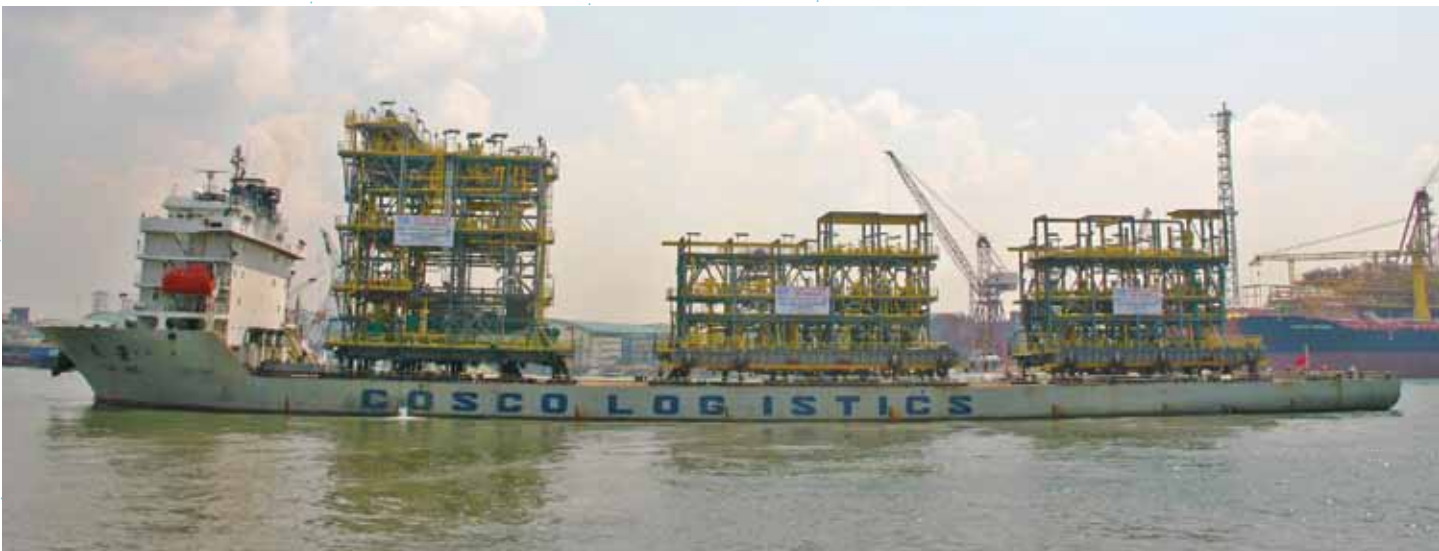
The loaded-out modules transported by floating barge to location
