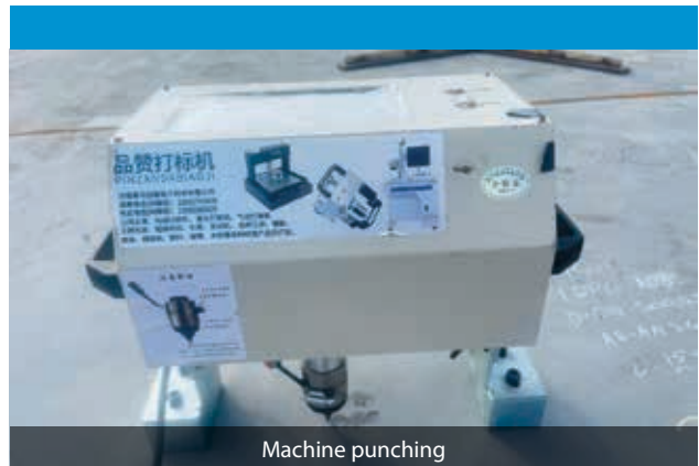
Setting of the Auto hand-held auto metal marking machine
